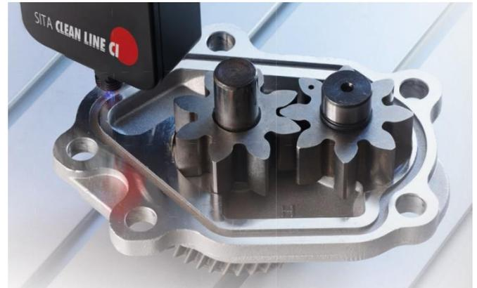
Figure 2: In-line cleanliness inspection of the sealing groove
