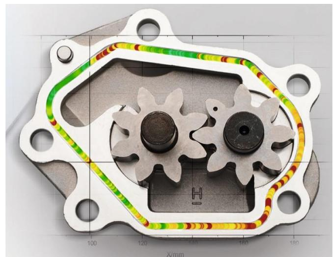
Figure 3: Colour-coded visualisation of the in-line inspection results
