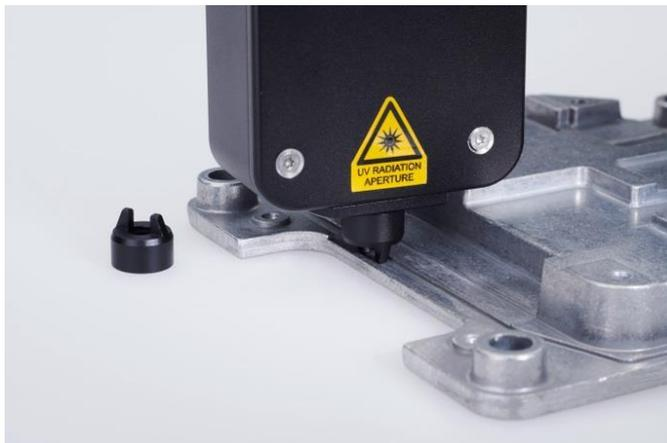
Figure 1: Manual measurement with SITA CleanoSpector and spacer directly on the adhesive groove
