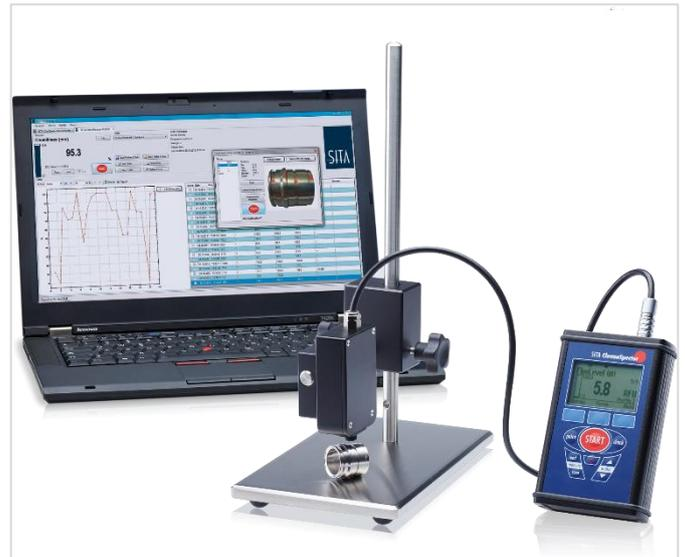
Figure 3: Mobile measuring device SITA CleanoSpector
